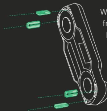
When you release the connector from the bottle, be careful not to lose the four „bumpers“. Should a bumper come loose, simply push it back into the relevant corner of the connector.
